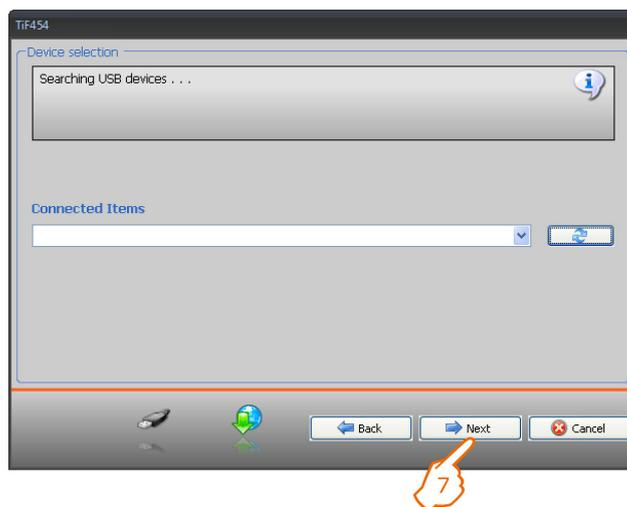
6. Wait for the device to be recognised automatically.
