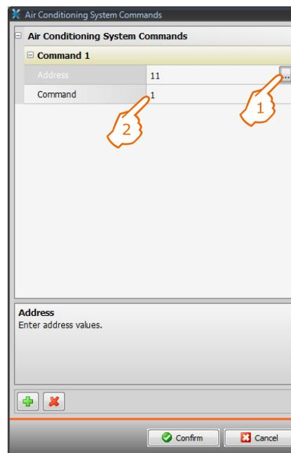
1. Enter the 3456 interface address (see "Common Configurations" ).
