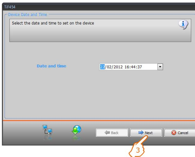
3. Click Next to display the window for the selection of the mode of connection with the device. The sending operation can be performed using two different types of connection:
