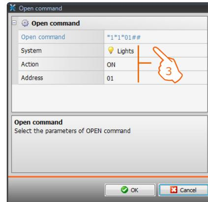
3. Automatically define the command to block by selecting in the appropriate screen: the system (Scenarios, Lights or Automation), the action (which changes depending on the system) and the SCS address (see "Common Configurations" ).
