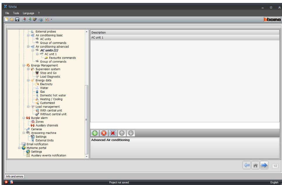
This window can be used to configure the parameters of the AC unit.
